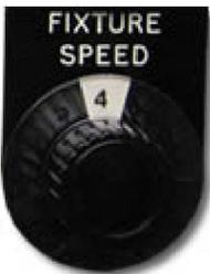
A D.C. thyristor drive control provides the variation in speed of the rotary fixture, for both the Fixed and Variable Machines. The fixture speed sets the feed rate which the samples are machined.
